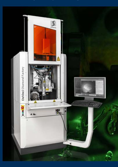
DaVinci system). The system is equipped to import third party software used for scanning the stone and planning for optimized use. After carrying out an optical alignment to establish a centre point in the cut stone, it first shapes the facets on the pavilion. This is where the laser beam can cut off large diamond chips that can be used for
