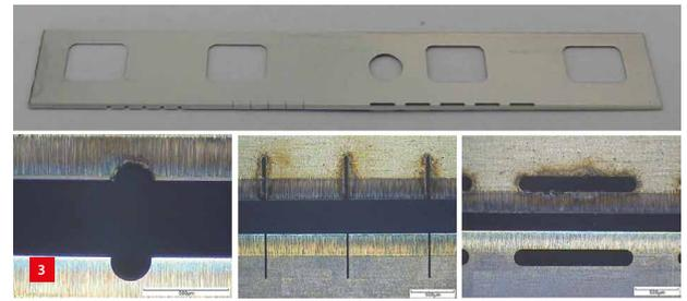
Below a stainless-steel shaver blade, three comparisons of cutting quality between conventional laser (middle row) and LMJ (bottom row) processing. (Image credit: Synova)
