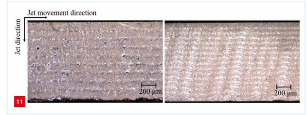
Comparison of the kerf surface of a 1.4-mm-thick silicon sample machined with the multi-pass strategy; left and right with different laser power and process speed values (see the text).
