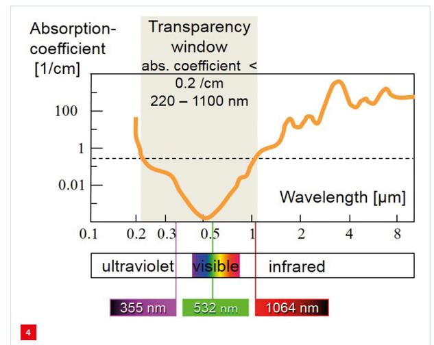
Water absorption spectrum from UV to IR wavelength. (Image credit: Synova)
