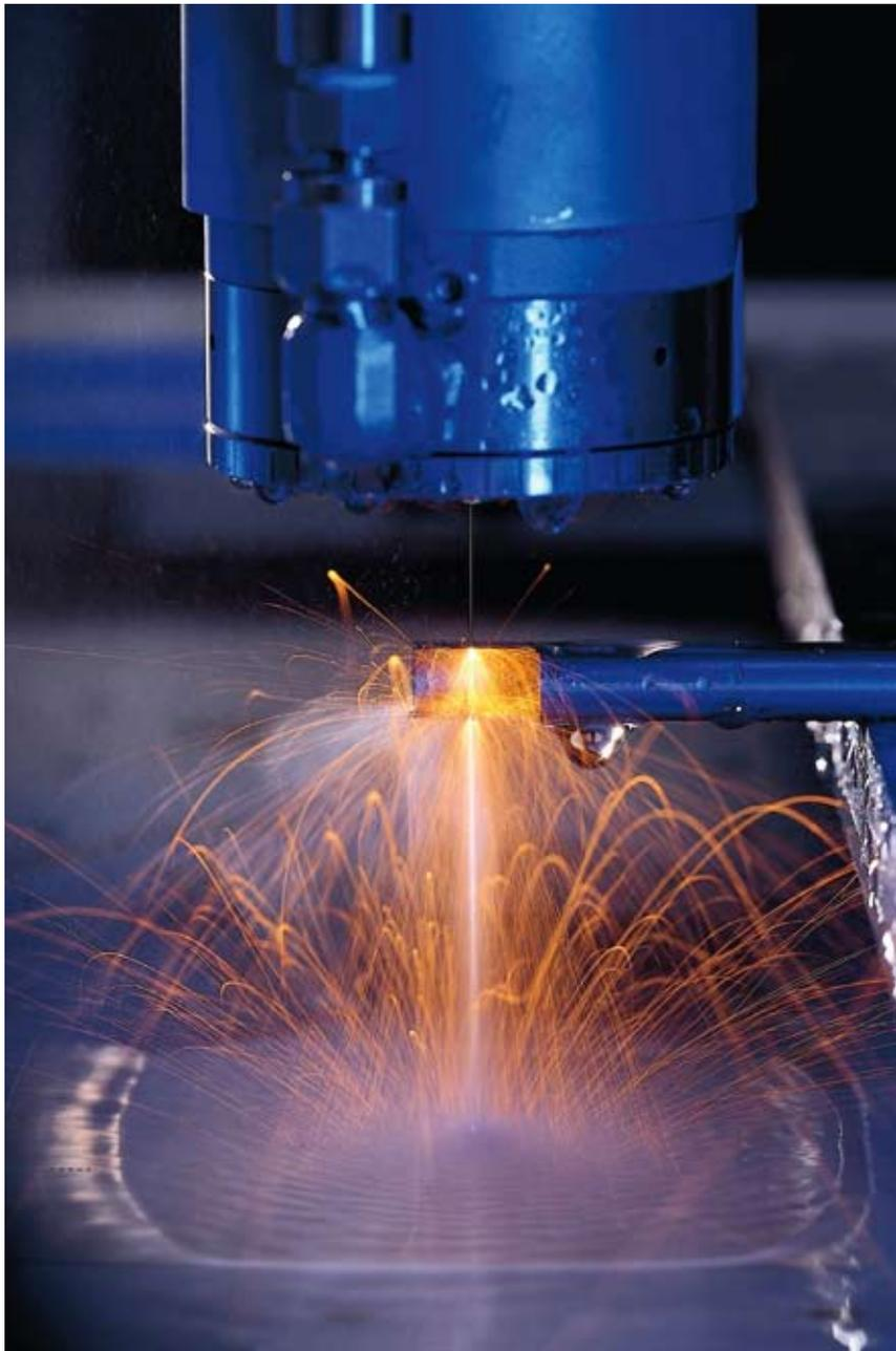
**Laser Microjet in operation: the waveguide principle of the water jet guides the pulsed laser beam to the workpiece. The cut edges are perfectly parallel to the water jet. The water jet has a cooling effect on the workpiece while cutting.**
