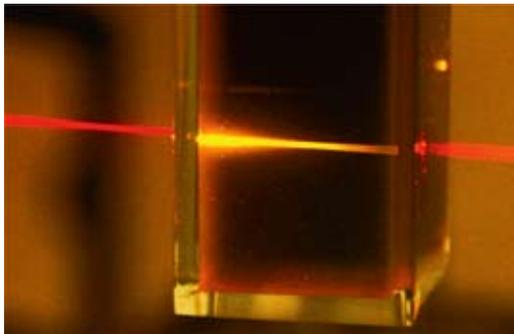
**Turbocharged cell: the red light from a laser pointer is converted to higher-energy yellow light on passing through the photochemical upconverter liquid.**
