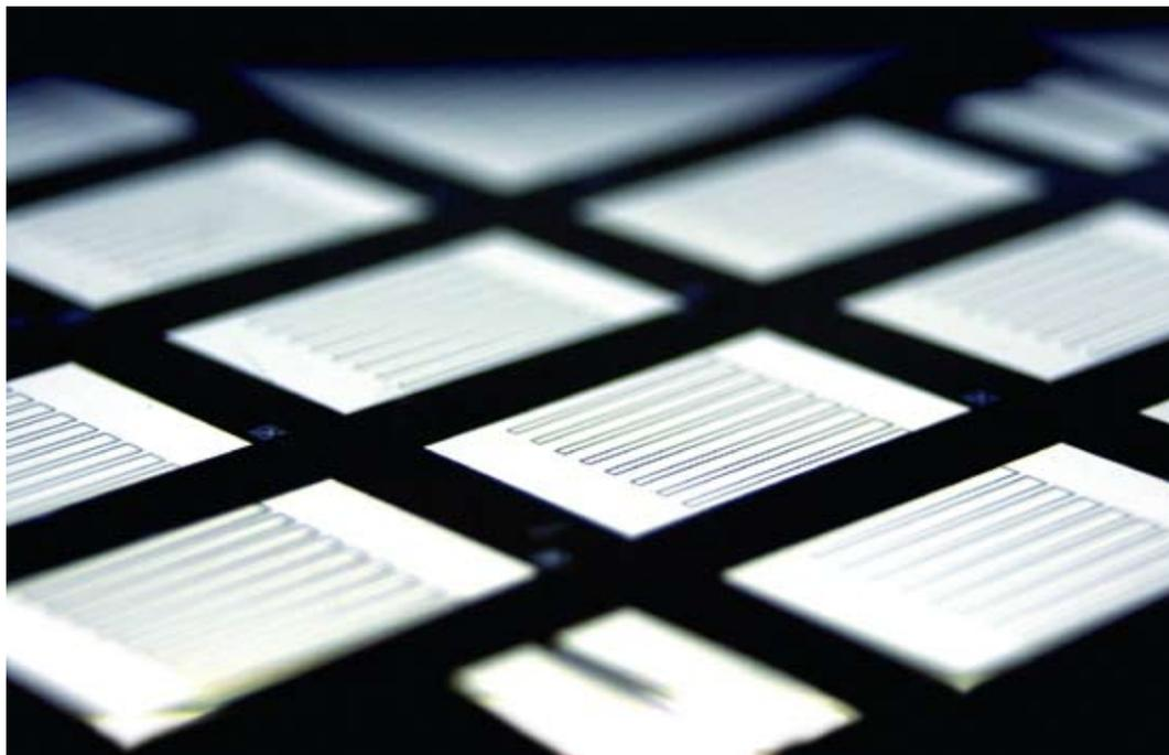
Back hetero: comb-shaped interlocking metal contacts on the back of rear-side solar cells with silicon heterocontacts. Several test cells on a silicon wafer can be seen.
